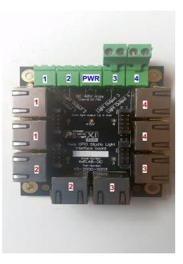
There are 2 RJ45 connectors for each of the 4 lights, they are just connected in parallel, so it doesn't matter which of the 2 you connect to. It's built that way to allow the GPO cable to be looped through to something else, or around to another input where the jumper is set to a different pin. With Pathfinder you could use 1 port (different pins) to trigger 4 lights by just looping it around through all 4 ports.
