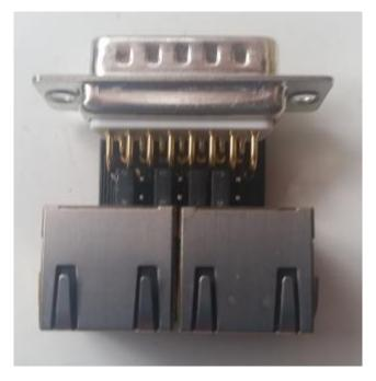
The board consists of a single DB15 male and two RJ45 sockets as pictured. There is a series of jumpers that must be set depending on how the board is to be used. As shown above Pin 1 is on the right-hand side.
